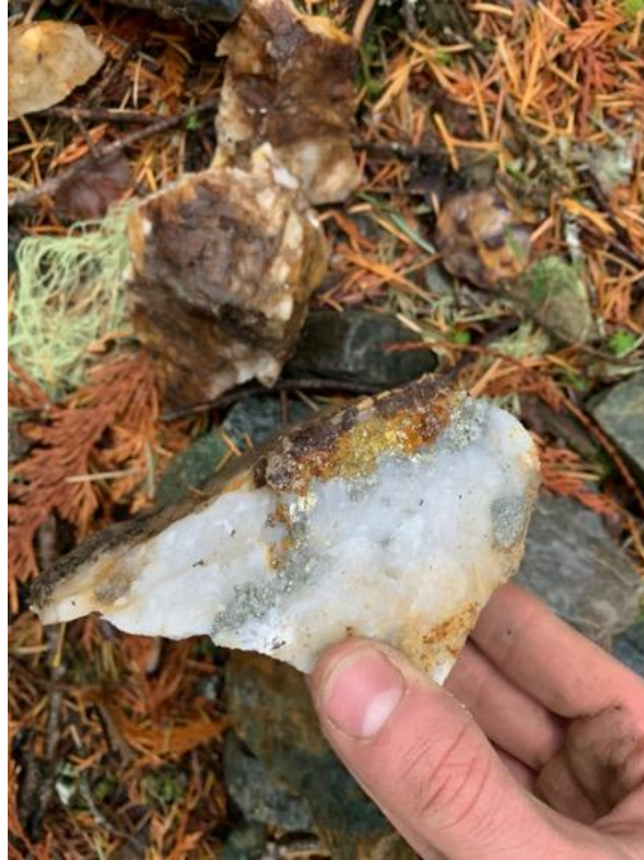
Quartz mineralized with pyrite from Good Hope prospect that assayed 2.82 grams per tonne gold.
