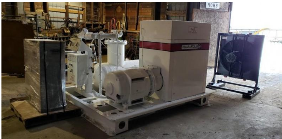
Compressor #1 on site at the Kenville Gold Mine. 600 v, 200 hp, 1000 cfm, extra high efficiency. Its' ready and waiting.
