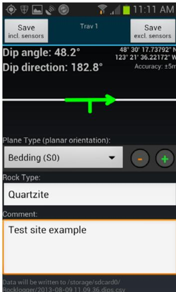
**Rocklogger screen capture of typical structural orientation entry page.**
