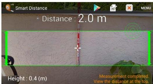
***Smart Distance* screen capture showing example of measuring distance utilizing an object of known height, in this case a Yamayo Model C Mini-Rod pocket stadia.**
