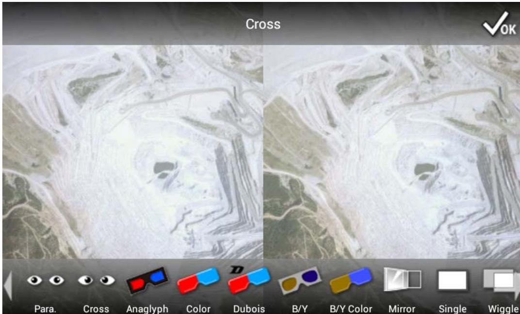
**Cross-eyed stereo view of a Highland Valley pit made using free downloaded colour airphotos from GeoBC. Cross your eyes to view in stereo.**
