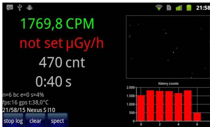
***Radiation Counter* screen capture showing sensing page.**
